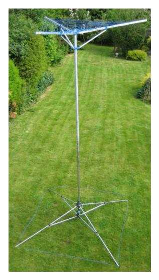
I used three wire spirals in this design which made it resonant at around 5MHz, however I intend to change this to just one long spiral, which should make it tune directly on 3.6MHz. Here's a closer view of the spiral top loading coil.
