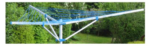
In order to bring it to resonance on 80m, I had to cut the aluminium support tube at the base and insert a short length of PVC water pipe to add a matching coil.
