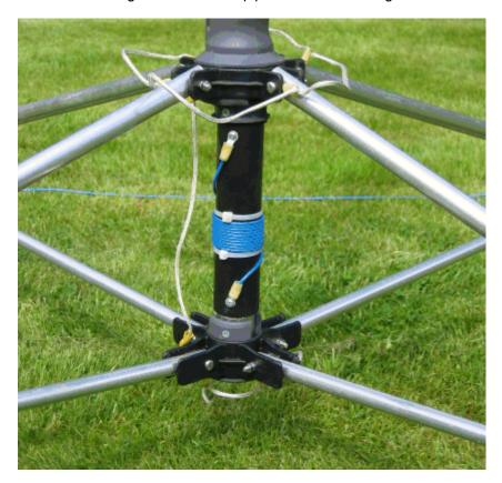
Note the bonding straps made from coax braid which I added to ensure all the metal bits were at the same potential.
