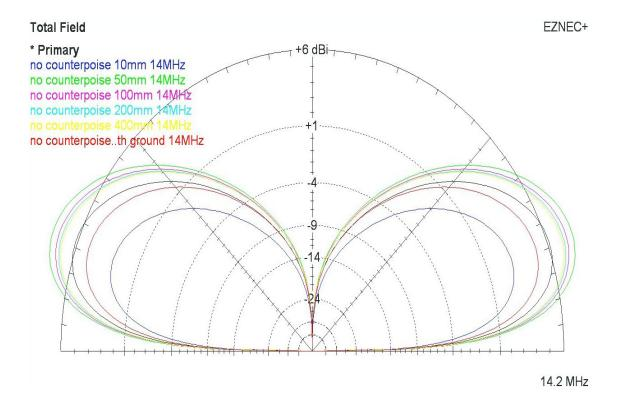
The results are highly suspect, as only a few mm differences in wire length make a large difference in gain approx +/- 3dB.
