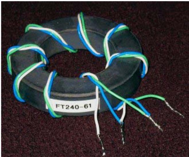
Finally achieved good bandwidth 1.8 to 30MHz with less than 0.5dB loss.
