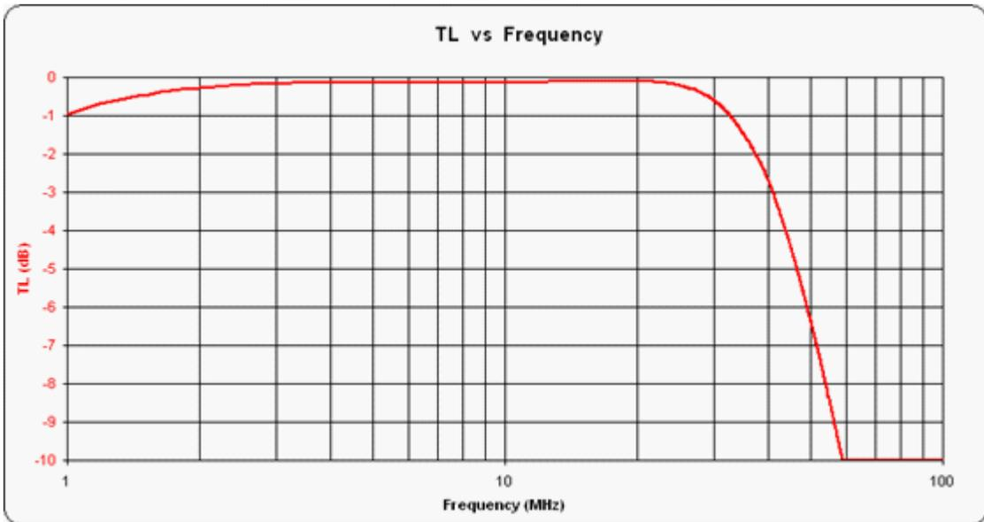
Second attempt at Unun, further optimised with 6 trifilar turns of 18AWG silver plated stranded wire. PTFE insulation, 1.85mm outer dia (CPC part number [CB10433](#)) wound on FT240-61 core.
