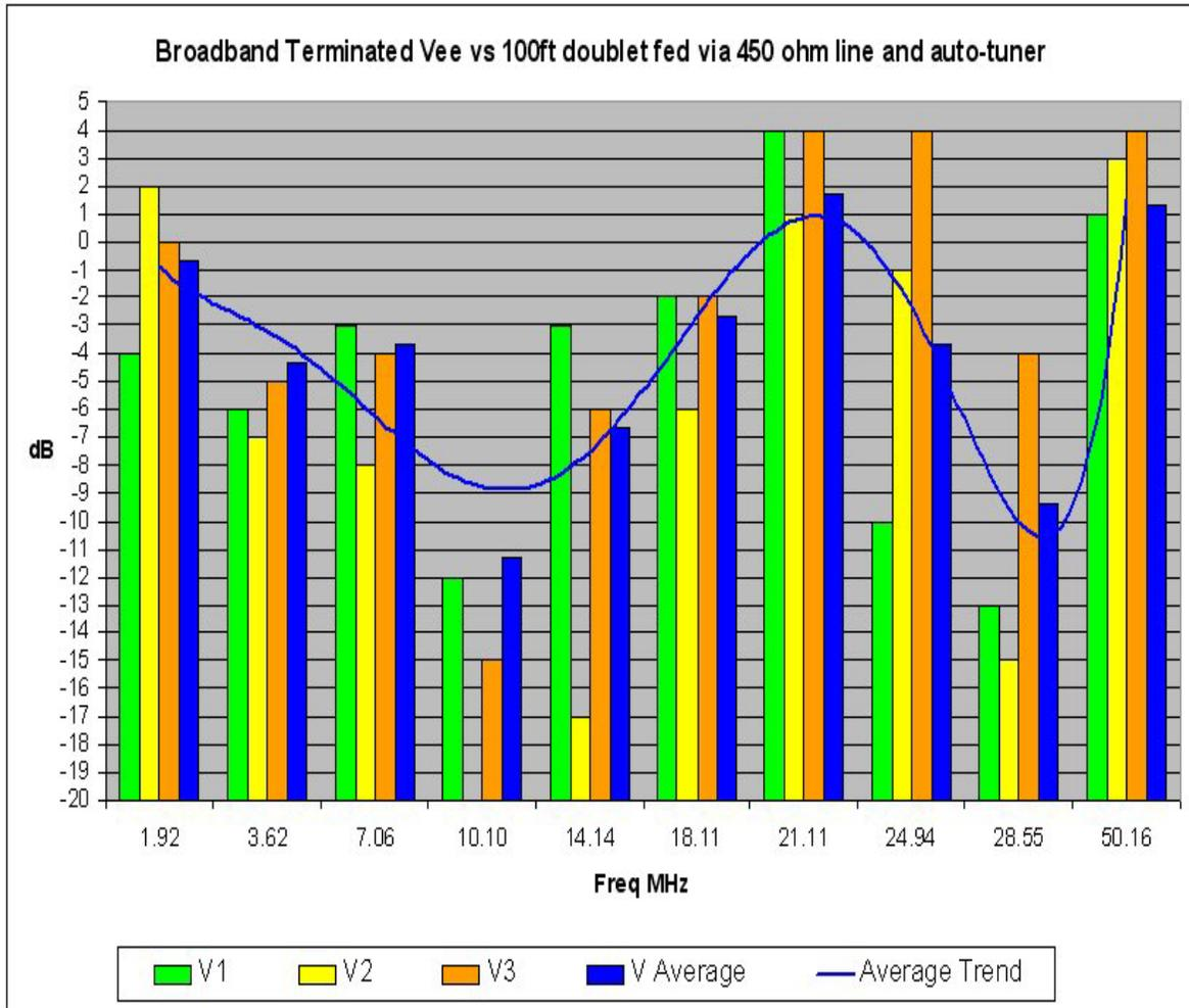
V1 is firing N-S, V2 is reversed firing S-N and V3 is like V1 but with one leg moved 30 degrees in order to try and gauge the directivity of the antenna.
